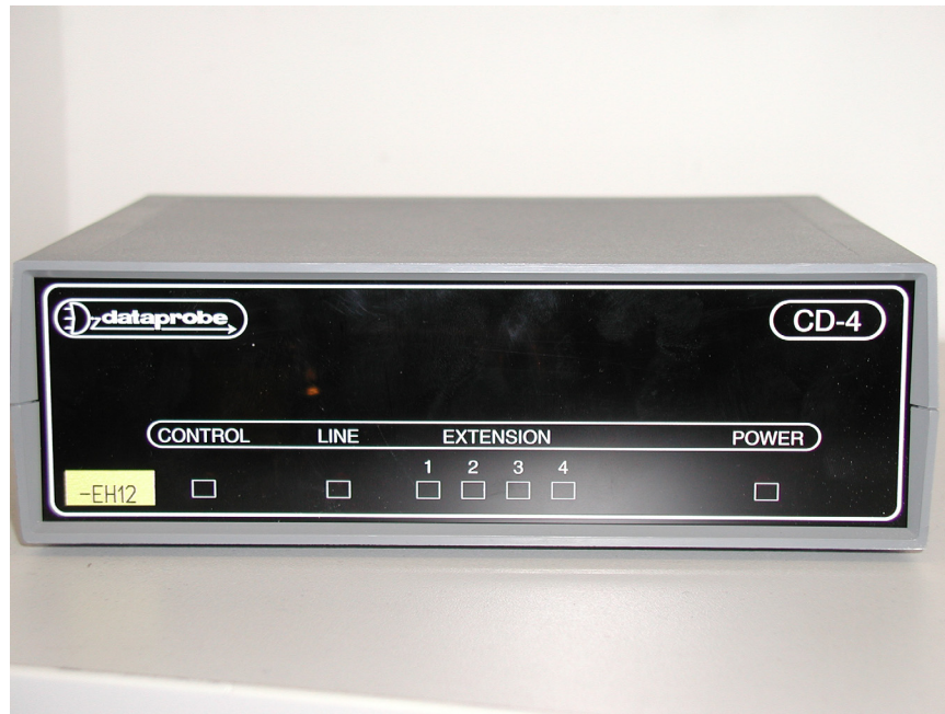
Figure 22: Front view of a modem splitter with four outputs by company dataprobe
