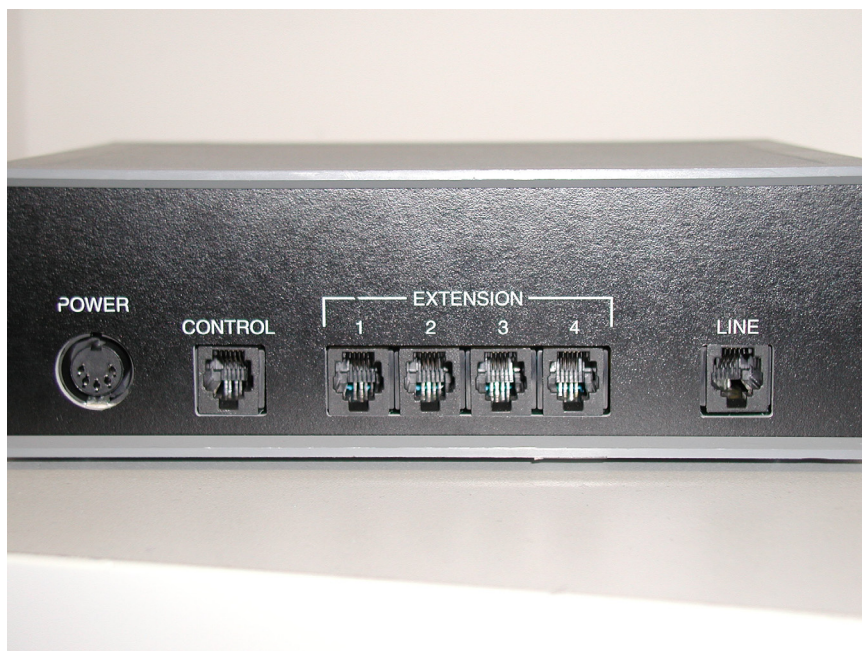
Figure 23: Rear view of a modem splitter with four outputs by company dataprobe
